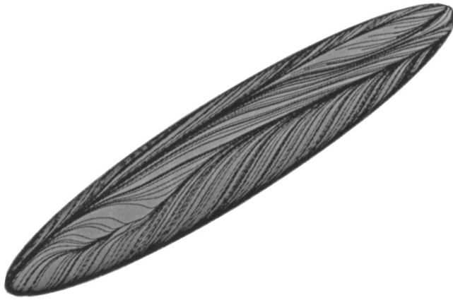
Fig. 2 Surface flows from DES prediction at 20 deg angle of attack. Flow is tripped at x/L=0.2 .
